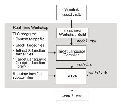
The Target Language Compiler (TLC) is designed for one purpose — to convert the model description file <code>model.rtw</code> (or similar files) into target-specific code or text.
