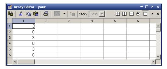
Column 1 contains discrete pulse output for six time steps (3s and 0s), collected at port out1.
