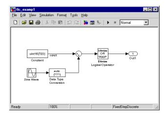
The code generated for the bit-wise operator block reuses a temporary variable that is set up for the output of the sum block to save memory. This results in one very efficient line of code, as seen here.
