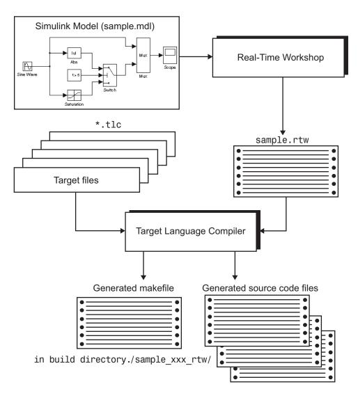
When generating code from a Simulink model, the first step in the automated process is to generate a <code>model.rtw</code> file. The <code>model.rtw</code> file includes all the model-specific information required for generating code from the Simulink model. <code>model.rtw</code> is passed to the Target Language Compiler, which uses it in combination with a set of included system target files and block target files to generate the code.
