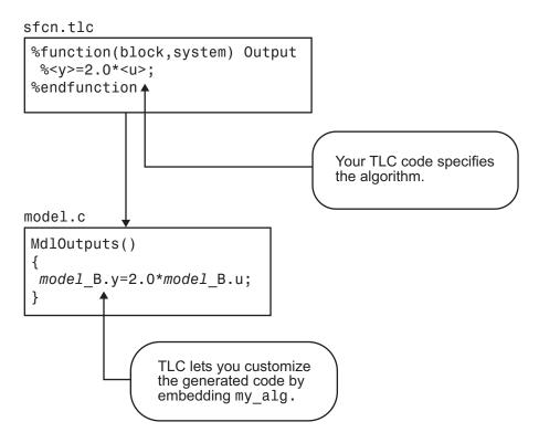
The S-function timestwo.c provides a simple example of a fully inlined S-function. This block multiplies its input by 2 and outputs it. The C MEX version of the block is in <code>matlabroot/simulink/src/timestwo.c</code>, and the inlining TLC file for the block is in <code>matlabroot/toolbox/simulink/blocks/tlc\_c/timestwo.tlc</code>.
